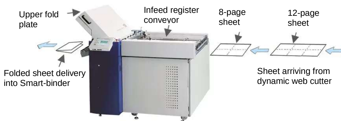
F-200 folder cross-folder unit used directly before SB infeed
