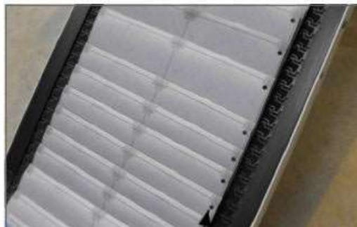
Booklets with punched holes on trimmer delivery conveyor
