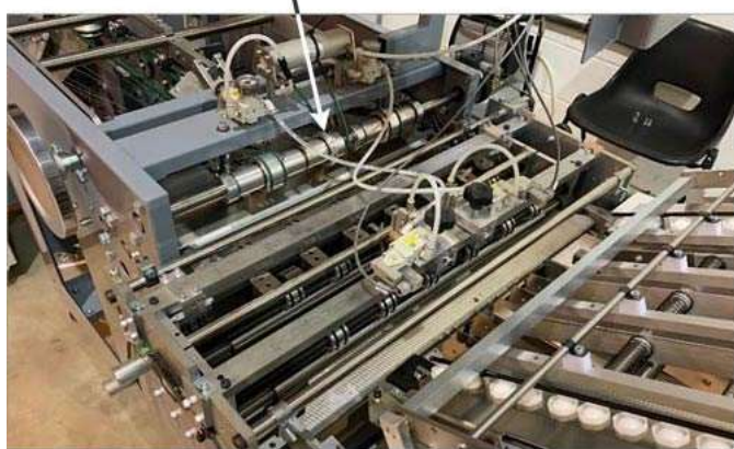
DMP-100 Rotary perforator knife actuators
