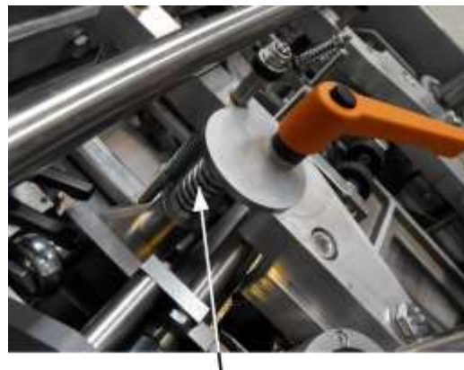
Hole punch installed in trimmer
