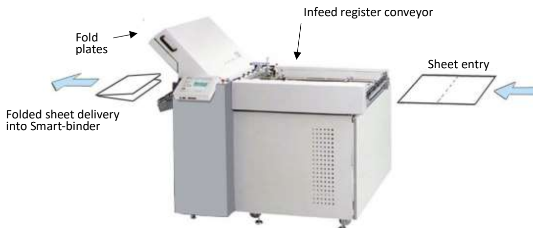
F-100 cross-folder unit used directly before SB infeed
