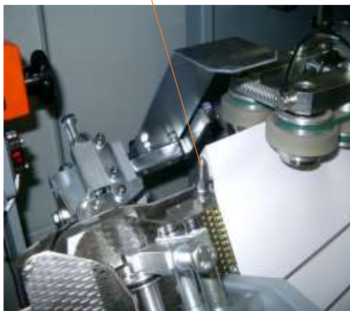
ISG Cold-Glue Application Nozzle on the Smart-binder
