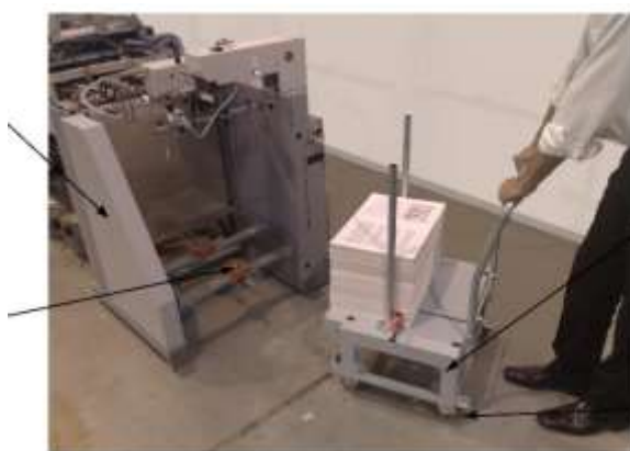
Trolley used to transport sheets to the pile feeder
