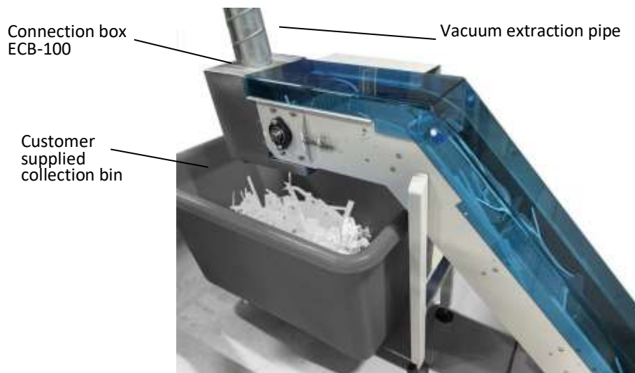
Vacuum extraction system via ECB-100 connection box, with lower bin
