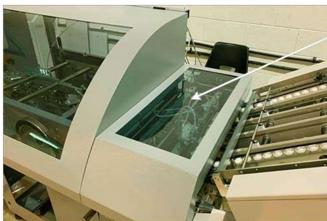
DMP Dynamic Perforation Unit mounted between the infeed conveyor and the scoring module
